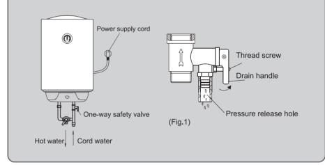
When using the heater for the first time(or the first use after maintenance), the heater can not be switched on until it has been filled fully with water. When filling the water, at least one of the outlet valves at the outlet of the heater must be opened to exhaust the air. This valve can be closed after the heater has been filled fully with water.
