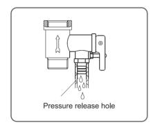
The drainage pipe connected to the pressure release hole must be kept sloping downwards.
